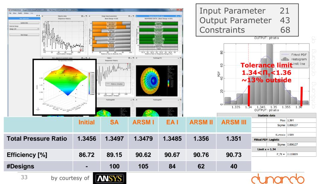
Robust Design Optimization with respect to 21 design parameters and 20 random geometry parameters, including manufacturing tolerances. Robust Design was reached after 400+250=650 design evaluations.
