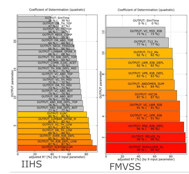
The coefficients of determination of the folded airbag analysis show significantly lower values ⇒ in this case it could be shown that the folded airbag does have much more numerical noise than the unfolded!
